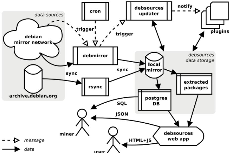
*In essence, Debsources does the **heavy lifting** of maintaining a general purpose [always up to date] storage for Debian source code, enabling plugin authors to focus on **data extraction**.*
