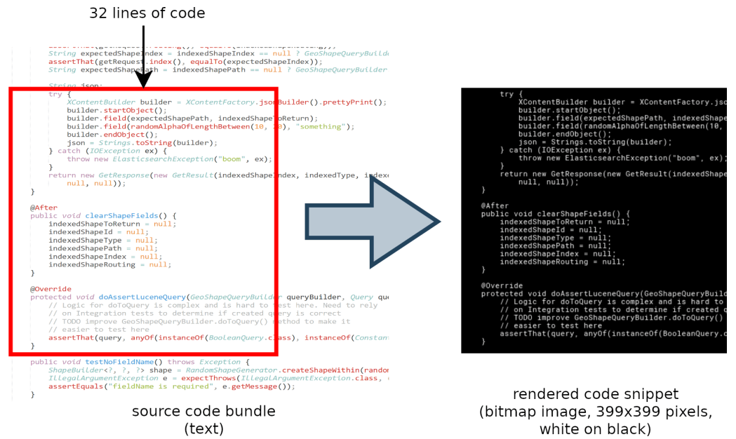
Figure 1 Source lines of code extraction from source code bundles and their rendering.
