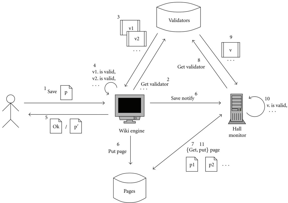
FIGURE 3: Runtime behaviour of the Save action.
